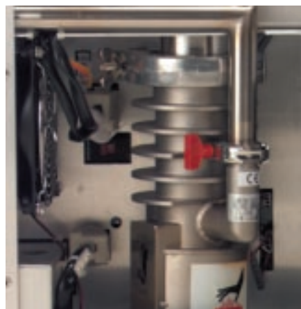
Saturn 2100D The Varian AX-65 diffusion pump provides high efficiency vacuum at the lowest possible cost. The custom-built Peltier cooler assures contamination-free vacuum.
